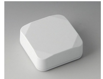
B1804217 MINI-DATA-BOX S50, high ASA+PC (UL 94 V-0) traffic white RAL 9016 50x50x20mm IP 65 opt., IP 40
