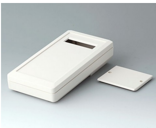
A9074307 DATEC-MOBIL-BOX M, Vers. III ABS (UL 94 HB) off-white RAL 9002 195x101x44mm IP 65 opt.
