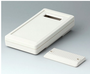
A9073307 DATEC-MOBIL-BOX S, Vers. III ABS (UL 94 HB) off-white RAL 9002 152x83x33.5mm IP 65 opt.
