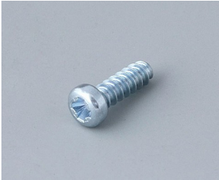
A0325080 Self-tapping screws 2.5 x 8 mm (PZ1)
