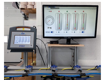
Monitoring system for cleaning nozzles
