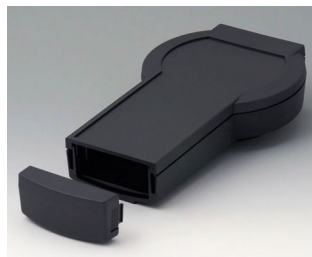
A9079109 DATEC-CONTROL L, Vers. I ABS (UL 94 HB) black RAL 9005 266x144x60mm IP 54 opt.
