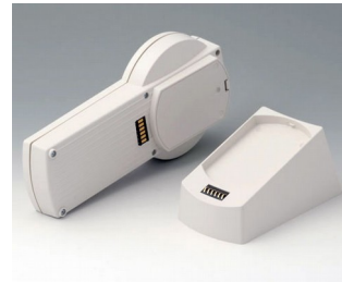
A9077257 SET: DATEC-CONTROL S, Vers. II, station.. ABS (UL 94 HB) off-white RAL 9002 228x117mm IP 65 opt.
