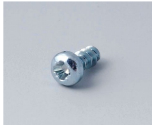
A0305031 Self-tapping screws 2.5 x 6 mm (PZ1)
