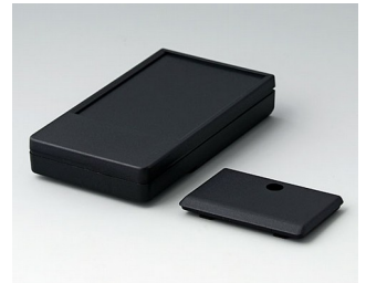
A9071219 DATEC-POCKET-BOX M ABS (UL 94 HB) black RAL 9005 105x58x18.5mm IP 54
