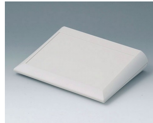
A0620007 COMTEC 200 F, Vers. I ABS (UL 94 HB) off-white RAL 9002 200x150x42.8mm IP 40
