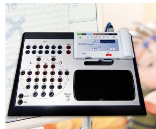
Stationary system for long-term EEG recordings
