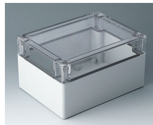
C7016064 IN-BOX ABS/PC (UL 94 HB) light grey RAL 7035 162x122x90mm IP 66, IP 67, IK 07
