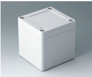
C7008021 IN-BOX ABS (UL 94 HB) light grey RAL 7035 84x82x85mm IP 66, IP 67, IK 07
