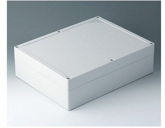
C7030102 IN-BOX PC light grey RAL 7035 302x232x90mm IP 66, IP 67, IK 08
