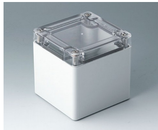
C7008024 IN-BOX ABS/PC (UL 94 HB) light grey RAL 7035 84x82x85mm IP 66, IP 67, IK 07
