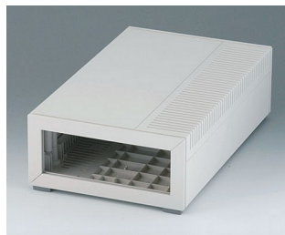
B2212007 MEDITEC E 220, without handle bar ABS (UL 94 HB) off-white RAL 9002 160x260x74mm IP 40
