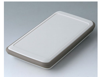
B5403217 SLIM-CASE M, Vers. V ASA+PC (UL 94 V-0) off-white RAL 9002 148x74x22mm IP 54
