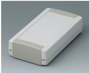
B1065365 TOPTEC 154 F, Vers. I ABS (UL 94 HB) off-white RAL 9002 154x84x38mm IP 40
