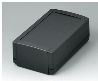
B1070369 TOPTEC 194 H, Vers. I ABS (UL 94 HB) black RAL 9005 194x115x68mm IP 40
