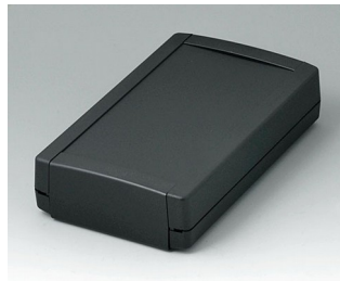
B1075369 TOPTEC 194 F, Vers. I ABS (UL 94 HB) black RAL 9005 194x115x46mm IP 40
