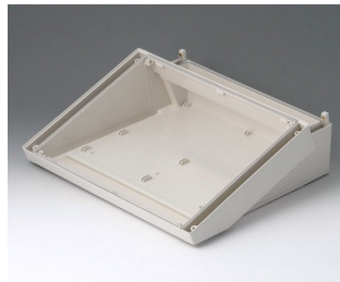
B4030117 DATEC-TERMINAL L, Vers. I ABS (UL 94 HB) off-white RAL 9002 302x272x101mm IP 54 opt.
