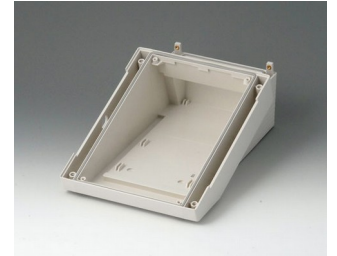
B4016317 DATEC-TERMINAL M, Vers. III ABS (UL 94 HB) off-white RAL 9002 168x272x101mm IP 54 opt.
