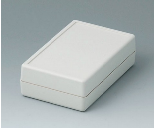
A9406351 SHELL-TYPE CASES G 110, Vers. I ABS (UL 94 HB) off-white RAL 9002 72x114x33.5mm IP 65 opt.
