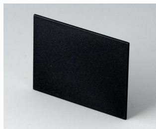
B6123222 Rear panel PPO (UL 94 V-0) black RAL 9005 63.8x49.2x1.7mm
