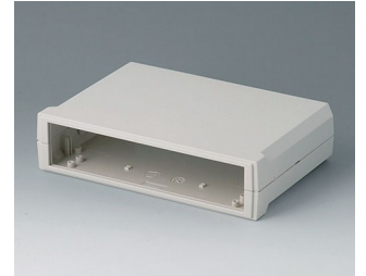
B3020117 MOTEC M, flat/flat ABS (UL 94 HB) off-white RAL 9002 205x140x50mm IP 40
