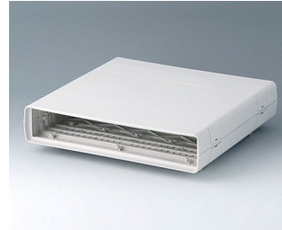
A0214070 EURO CASE 42 TE, without handle ABS (UL 94 HB) off-white RAL 9002 260x250x54mm
