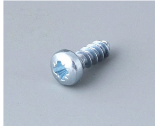
A0308031 Self-tapping screws 3 x 8 mm (PZ1)
