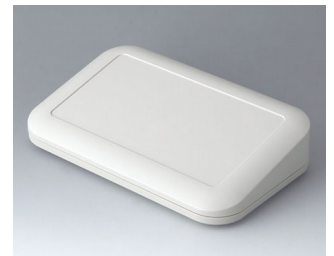
A9466107 EVOTEC 200, Vers. III ASA+PC (UL 94 V-0) off-white RAL 9002 200x124x45mm IP 65 opt., IP 40
