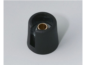
A3016069 COM-KNOBS 16, with recess PA 6 nero 16x16mm 6mm
