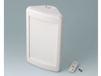
B4610207 SMART-CONTROL M, Vers. II ASA+PC (UL 94 V-0) off-white RAL 9002 173x101x59mm IP 55 opt., IP 40
