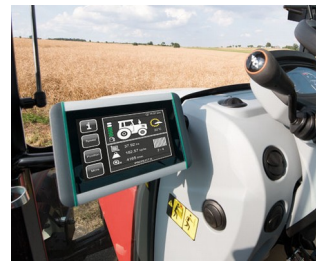
ISOBUS terminal for tractors and self-propelled machines
